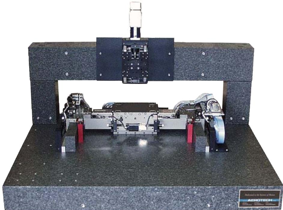
Shown is one example of a motion control platform intended to be used for non-contact surface profilometry. The system mechanics shown feature air-bearing motion to reduce motion-induced flatness errors, and a linear-motor vertical axis provides automated focus of the light-based sensor used for data collection. *Source: Aerotech Inc.*
