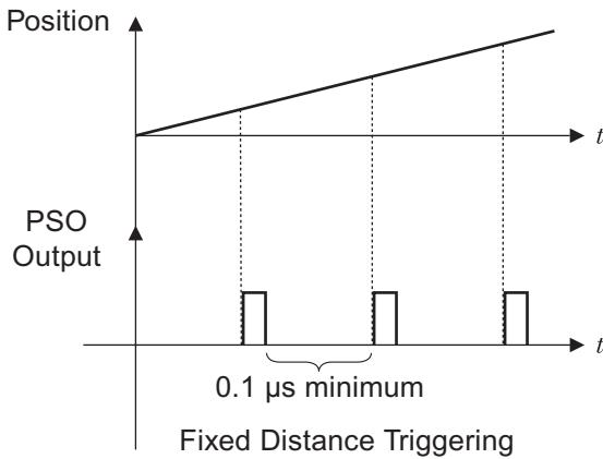
The most common means of implementing PSO in a testing application is to trigger the output pulse on a fixed distance. This method allows the operator to trigger a single pulse, or multiple pulses, at constant, prespecified intervals along the travel. The fixed-distance method is typically used to strobe the system's sensor to begin collecting data. Source: Aerotech Inc.
