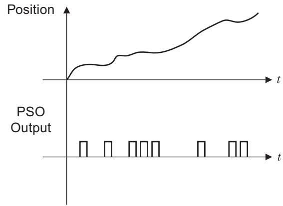
Array-based triggering allows the user to specify trigger points that are unequally spaced along the travel. This style of PSO firing can be used to trigger imaging sensors at precise positions for mapping or contouring operations, or perhaps when working with irregular part geometries. Source: Aerotech Inc.
