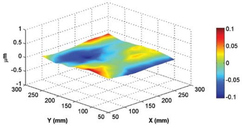
PSO triggering during continuous scans over the circular optical flat permits a number of sensor images to be collected at precise and, more importantly, well-known positions across and along the part. Because the positional data is trustworthy and tightly tied to sensor output timing, a contour map of the resulting image data can be easily reconstructed by stitching the data points together. *Source: Aerotech Inc.*
