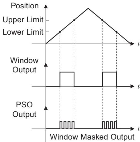
Windowing allows an input to be set when the axis is precisely within a specified position window. PSO provides up to two windows that can be used to specify two distinct areas of interest in one axis or for two-dimensional windowing. This functionality also can be coupled with fixed distance triggering to mask the triggering to certain areas of travel. This is particularly useful when direction reversals are required during large area scan routines. *Source: Aerotech Inc.*
