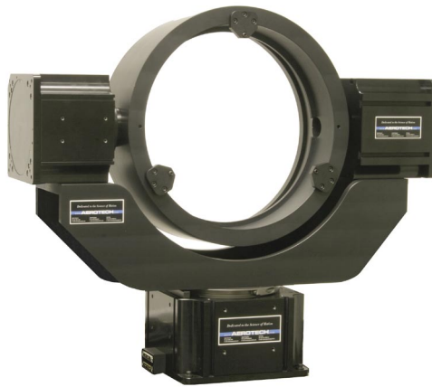
FIGURE 2. Compared to gear-driven gimbals, direct-drive gimbals offer higher accuracy and the ability to make quick movement and direction reversals. These attributes are useful for applications such as calibration and encoder testing, star and solar tracking, and inertial device testing.
